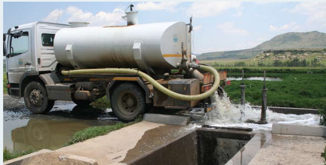
Sewerage Tanker at the discharge point at Ha Thetsane.
